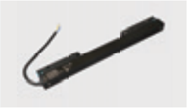
Magnetic power Model: JLY-EMC-20-200W48 Size: L365×W22×H44mm Input voltage: 220-240VAC Output: DC48V Power: 200W Applicable model: All staight track
